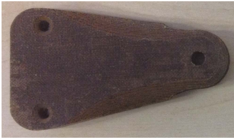
8: The triangular pulley insulator for the antenna wire and 9: the insulated, swivelling connector that was fitted to the rudder post [From http://spitfirespares.co.uk/radio.html ]
