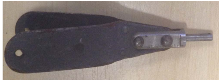
8: The triangular pulley insulator for the antenna wire and 9: the insulated, swivelling connector that was fitted to the rudder post [From http://spitfirespares.co.uk/radio.html ]
